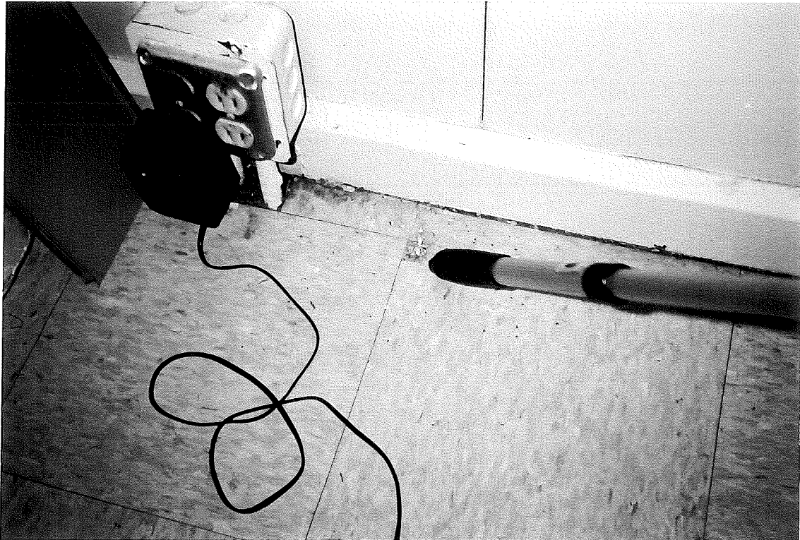
PHOTO 1: Negative Testing 12" Vinyl Floor Tile in Storage Area Overlies Asbestos-Containing Sheet Flooring (4)
