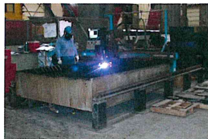
Plasma Table (right) utilizes computer accuracy to cut steel.
