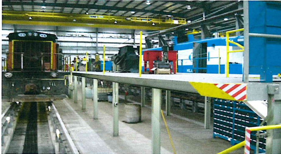
Cab angle view of RELCO's Raised Rails. RELCO's two state-of-the-art raised rails enable technicians easier access to work all around the locomotives. They also enable easier under-carriage inspections. All of this provides greater quality!
