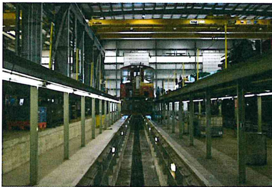
Below angle view of RELCO's Raised Rails; these also enable easier under-carriage inspections. All of this provides greater quality!
