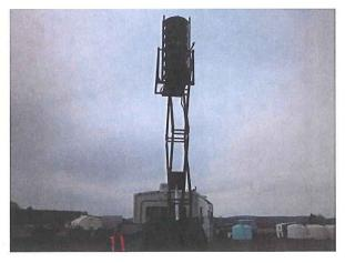
On 02-18-09 through 02-19-09, Crook County Emergency Management, the City of Prineville and the Bureau of Reclamation conducted field tests of an emergency alert system. The tests consisted of deploying a trailer mounted siren and public address unit at 7 key sites around the City, while personnel measured sound levels using sound pressure meters in various populated areas throughout the flood plain.
